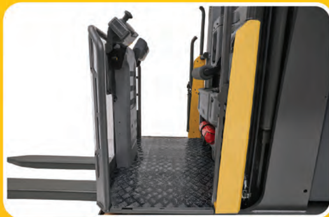
Cushioned, high-grip mat covers wholefloor driver presence sensor. Operation is permitted from any standing position. Walkthrough access is quick and free of tripping hazards, thanks largely to the absence of a traditional 'deadman pedal'.
